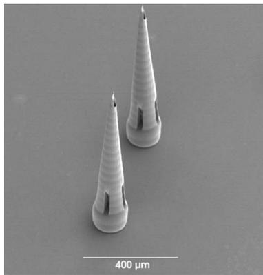
**Figure 1.24:** SEM image of micro-needles (Source: [www.belasnet.be](http://www.belasnet.be)<sup>9</sup>).
