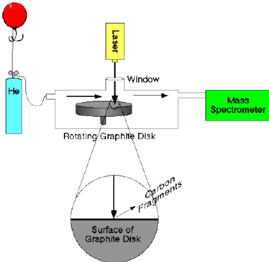
Figure 1.15: Smalley's apparatus<sup>6</sup>
