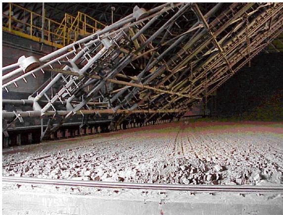
**Figure 4.32:** Raking device for reclaiming stored limestone (Copyright Halliburton Energy Services).
