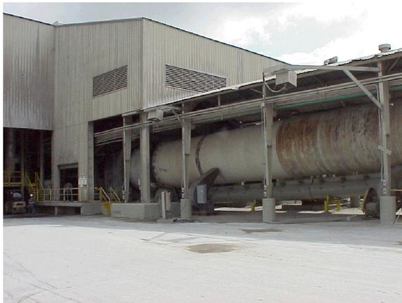
**Figure 4.35:** A wet rotary kiln (Copyright Halliburton Energy Services).
