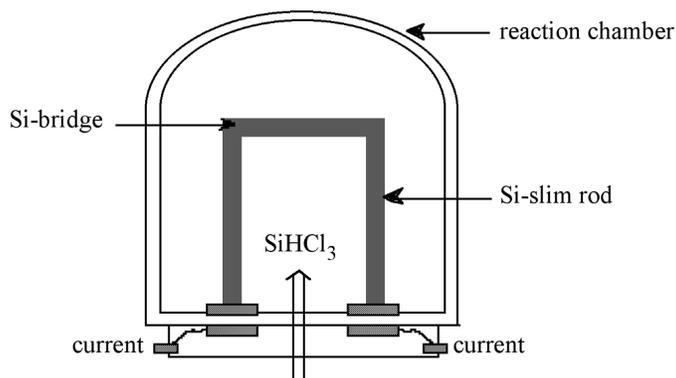
**Figure 3.2:** Schematic representation of a Seimens deposition reactor.
