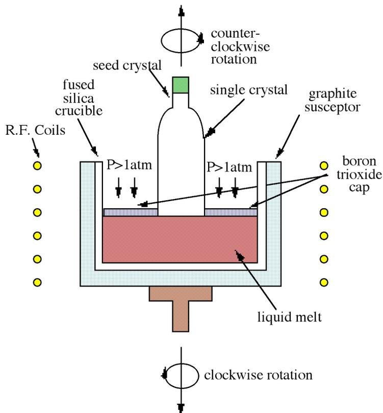
**Figure 3.7:** A schematic diagram of the Czochralski technique as used for growth of GaAs single crystal bond.
