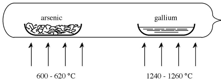
**Figure 3.5:** Schematic representation of a sealed tube synthesis of GaAs.
