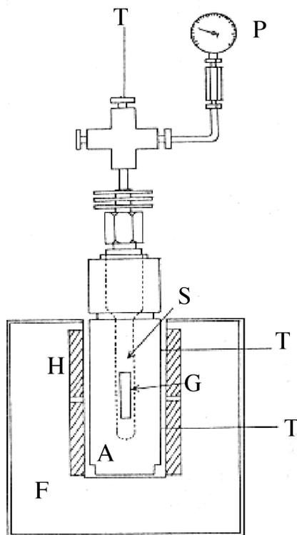
**Figure 3.9:** Experimental apparatus for the hydrothermal synthesis of barylite. H = heater, F = furnace, S = specimen vessel, G = growth capsule, P = pressure gauge, and T = thermocouples. Adapted from M. Maeda, T. Uehara, H. Sato and T. Ikeda, *Jpn. J. Appl. Phys.*, 1991, **30**, 2240.
