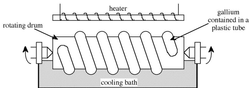
**Figure 3.4:** Schematic representation of a zone refining apparatus.
