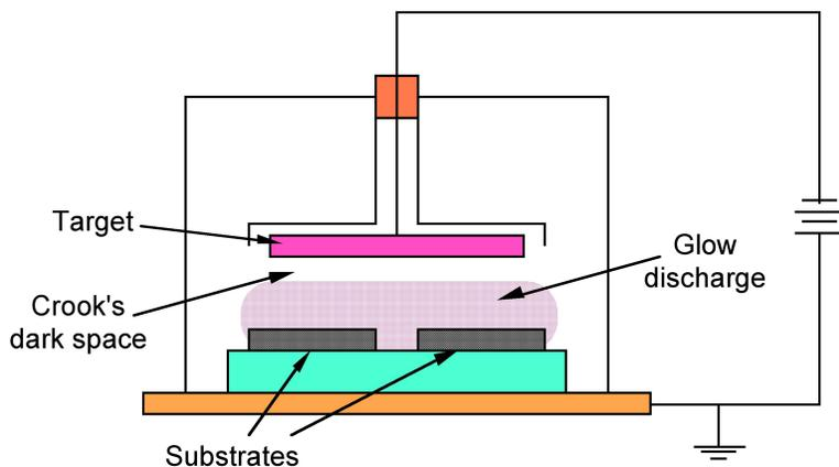
**Figure 4.42:** A schematic representation of a sputtering apparatus.
