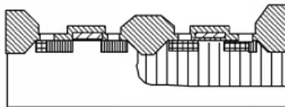
**Figure 4.41:** After the contact holes are etched.
