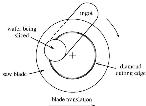
**Figure 4.5:** Schematic diagrams of ID slicing process.
