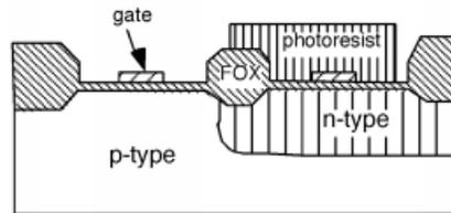
**Figure 4.35:** Preparing for NMOS channel/drain implant.
