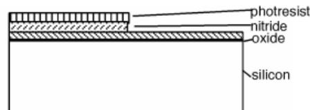
**Figure 4.22:** After the nitride etch step.
