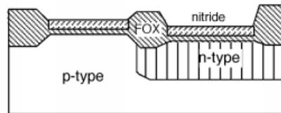
**Figure 4.32:** After growth of the field oxide (FOX).
