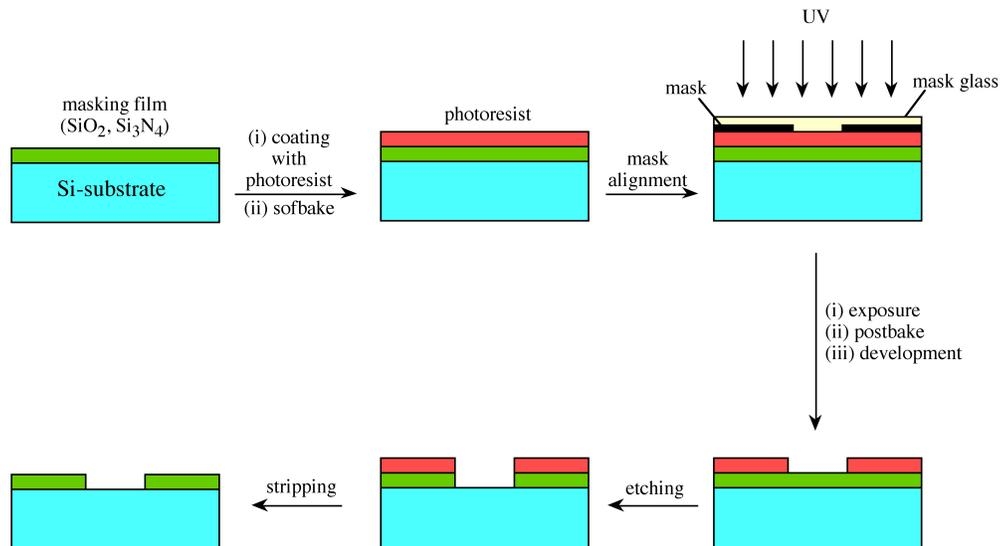
**Figure 4.24:** Steps in optical printing using photolithography.
