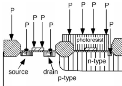
**Figure 4.36:** Phosphorus S/D implant.
