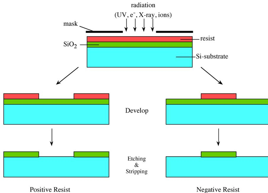
**Figure 4.27:** A comparison of negative and positive photoresists.
