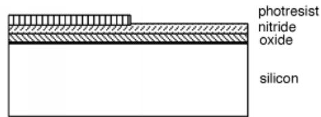
**Figure 4.21:** After photoresist exposure and development.
