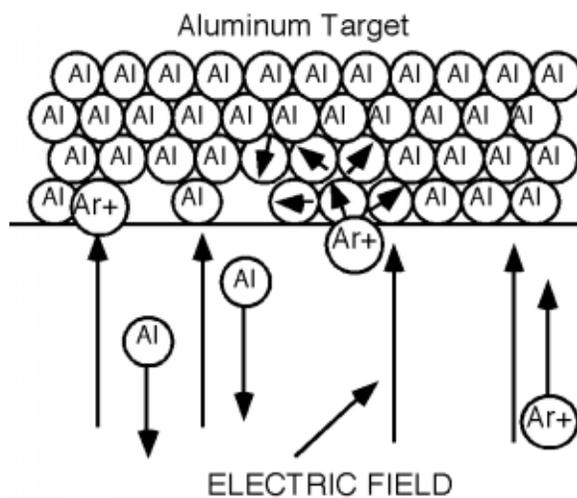
**Figure 4.43:** The sputtering mechanism.
