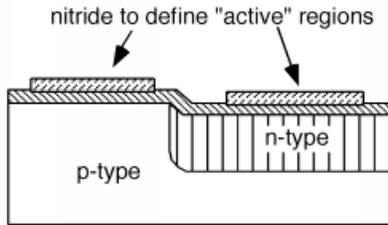
**Figure 4.31:** Nitride remaining after etching.
