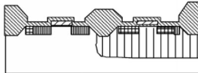
**Figure 4.40:** Final oxide growth.
