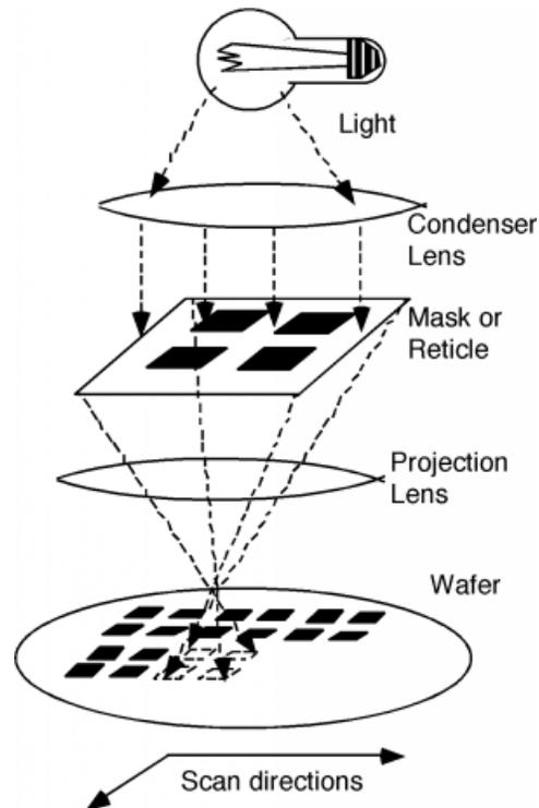
**Figure 4.20:** A schematic of a stepper configuration.
