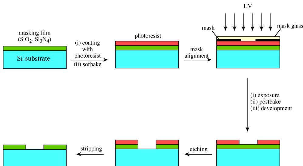
**Figure 4.25:** Steps in optical printing using photolithography.
