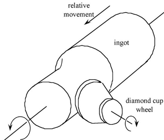
**Figure 4.2:** Schematic representation of grinding on center.
