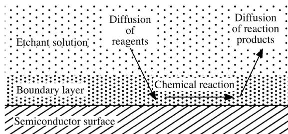
**Figure 4.7:** Schematic representation of the three steps involved in wet chemical etching: (i) diffusion of the chemical etch reagents through the boundary layer, (ii) chemical reaction at the surface, and (iii) diffusion of the reaction products into the etch solution through the boundary layer.
