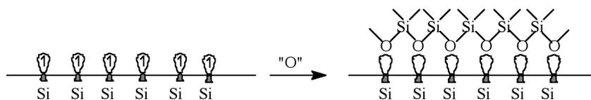
**Figure 4.15:** Removal of dangling bonds by oxidation of surface.
