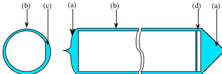
**Figure 4.1:** Schematic representation of crystal shaping operations: (a) remove crown and taper, (b) grind to required diameter, (c) grind flat, and (d) slice sample for measurements. Shaded area represents material removed.
