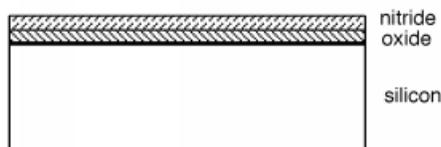
**Figure 4.18:** Initial wafer configuration.
