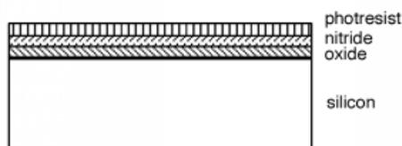
**Figure 4.19:** After the photoresist is spun on.
