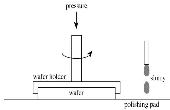
**Figure 4.11:** Schematic representation of the wafer polishing process.
