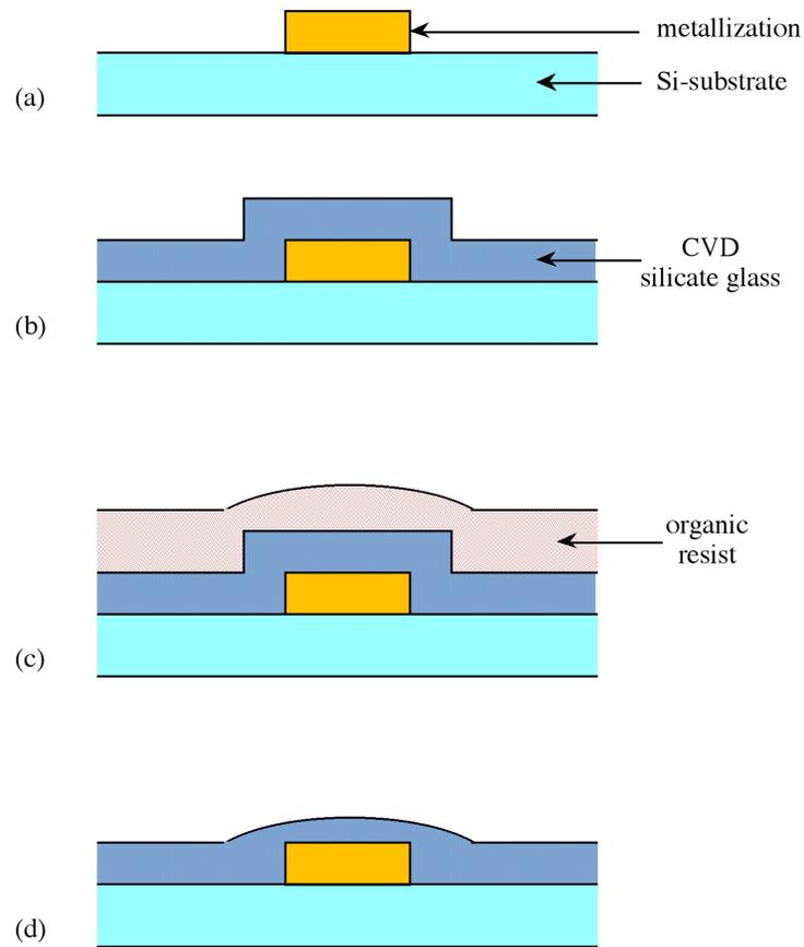
**Figure 4.14:** Schematic representation of the planarization process. A metallization feature (a) is CVD covered with silicate glass (b), and subsequently coated with an organic resin (c). After etching the resist a smooth silicate surface is produced (d).
