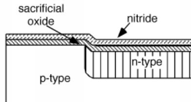
**Figure 4.30:** Strip of the oxide and grow a new nitride layer.
