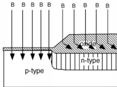
**Figure 4.29:**  $V_T$  adjust implant.
