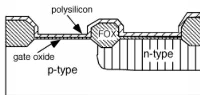
**Figure 4.34:** Polysilicon deposition over the gate oxide.
