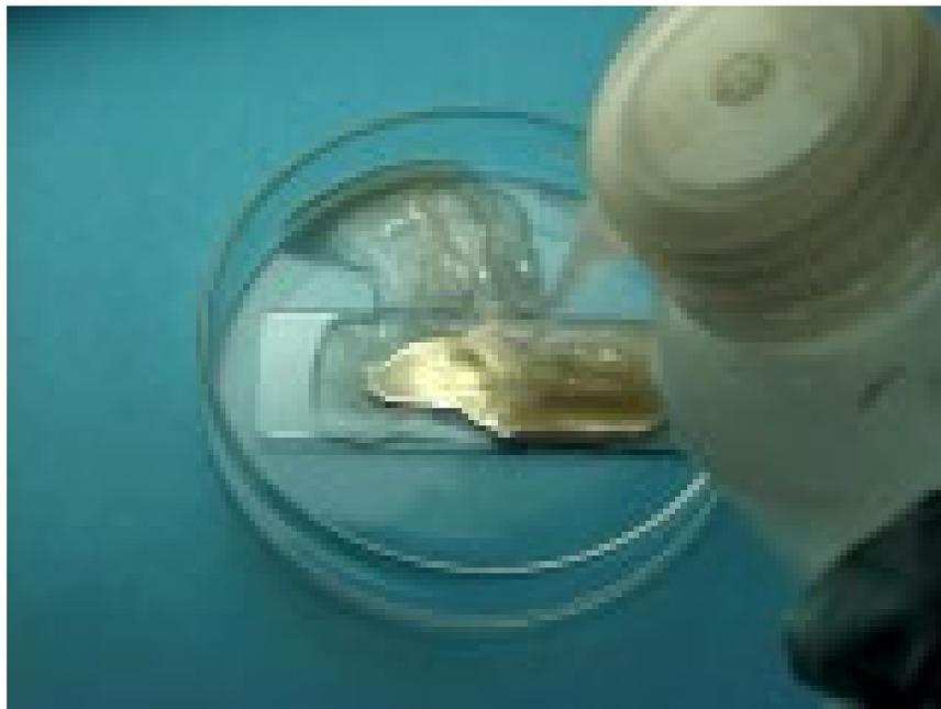
**Figure 2.24:** Image showing the silver mirror formed on the glass slide.
