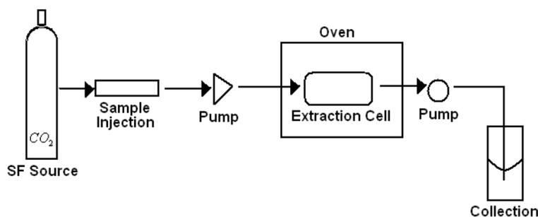
**Figure 4.23:** Scheme of an idealized supercritical fluid extraction instrument.
