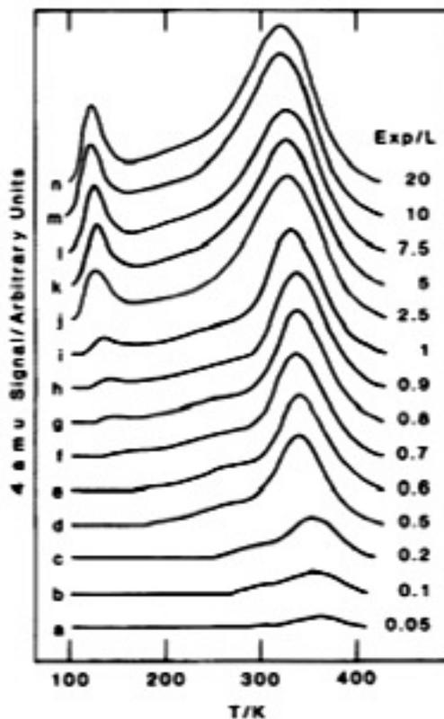
Figure 4.20: TPD spectra of  $D_2$  from Rh(100) for different exposures in L (1 Langmuir =  $10^{-6}$  Torr-s)<sup>6</sup>.
