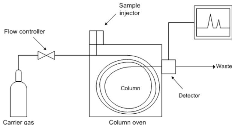
**Figure 4.1:** Physical components of a typical GC system. Adapted from [http://en.wikipedia.org/wiki/Gas\\_chromatography](http://en.wikipedia.org/wiki/Gas_chromatography)
