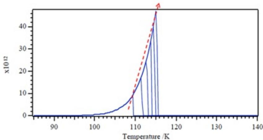
**Figure 4.19:** A simulated zero-order TPD experiment: A zero-order reaction between adsorbates and surface. Values of  $T_m$  increase apparently as the initial coverage  $\theta$  increases from  $1.0 \times 10^{13}$  to  $6.0 \times 10^{13}$   $\text{cm}^{-2}$ ;  $E_a = 30$  KJ/mol;  $\beta = 1.5$   $^{\circ}\text{C/s}$ ;  $A = 1 \times 10^{28}$ .
