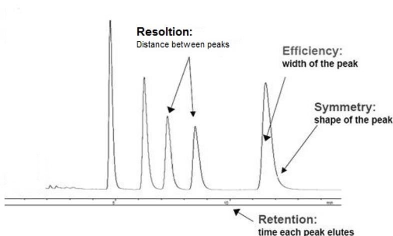
Figure 4.4: Separation terminology. Adapted from <http://www.gchelp.tk>
