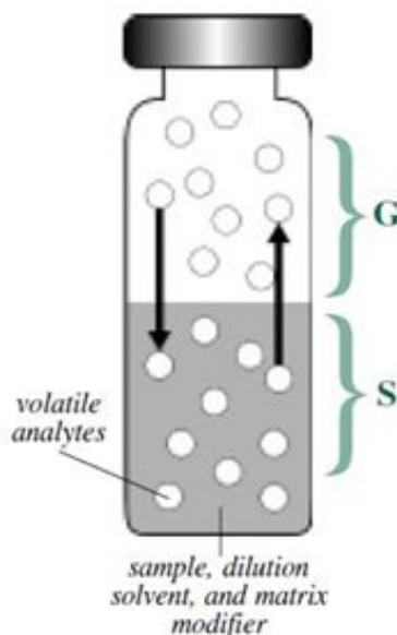
**Figure 4.10:** Schematic representation of the phases of the headspace in the vial. Adapted from *A Technical Guide for Static Headspace Analysis Using GC*, Restek Corp. (2000).
