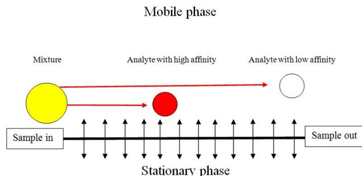
**Figure 4.9:** Scheme for partition in mobile and stationary phases.
