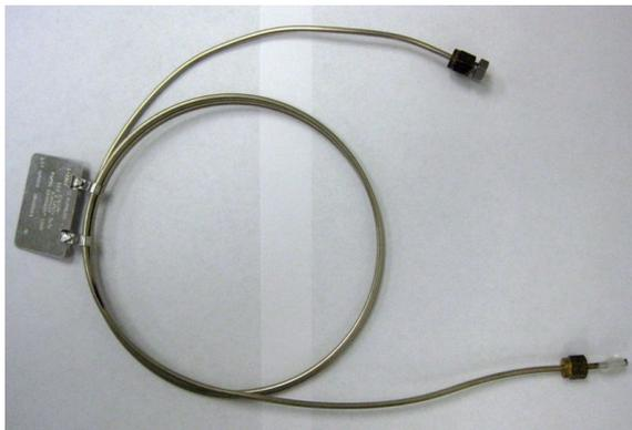
**Figure 4.2:** An example of a packed GC column.
