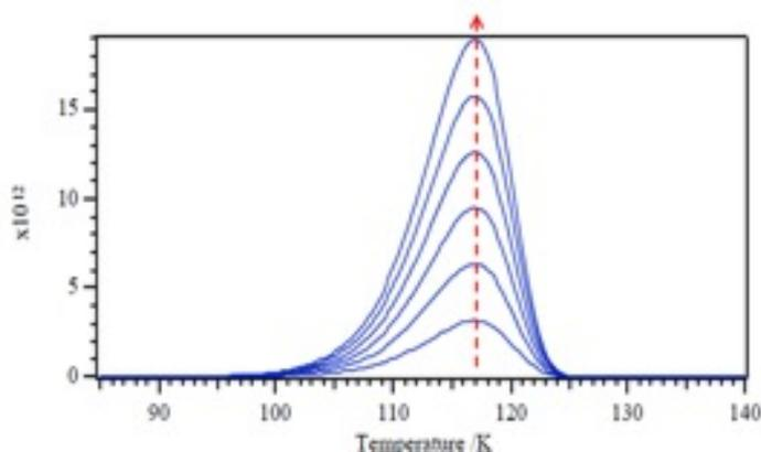
**Figure 4.17:** A simulated TPD experiment: Consider a first order reaction between adsorbates and surface. Values of  $T_m$  keep constant as the initial coverage  $\theta$  from  $1.0 \times 10^{13}$  to  $6.0 \times 10^{13} \text{ cm}^{-2}$ .  $E_a = 30 \text{ KJ/mol}$ ;  $\beta = 1.5 \text{ }^\circ\text{C/s}$ ;  $A = 1 \times 10^{13}$ .
