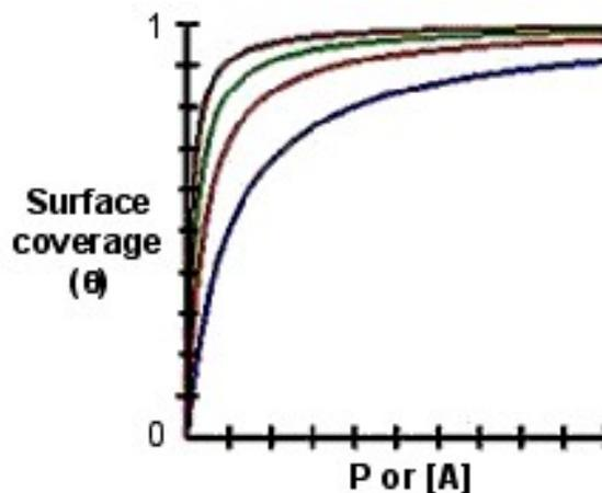
**Figure 4.16:** Simulated Langmuir isotherms. Value of constant  $K$  ( $k_a/k_d$ ) increases from blue, red, green and brown.
