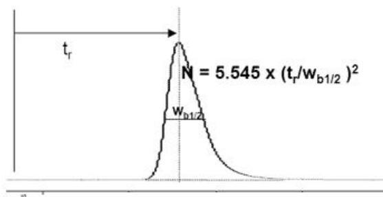
Figure 4.7: Scheme for calculating efficiency. Adapted from <http://www.gchelp.tk>
