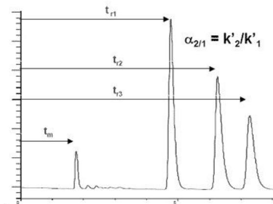
Figure 4.6: Scheme for the calculation of selectivity. Adapted from <http://www.gchelp.tk>
