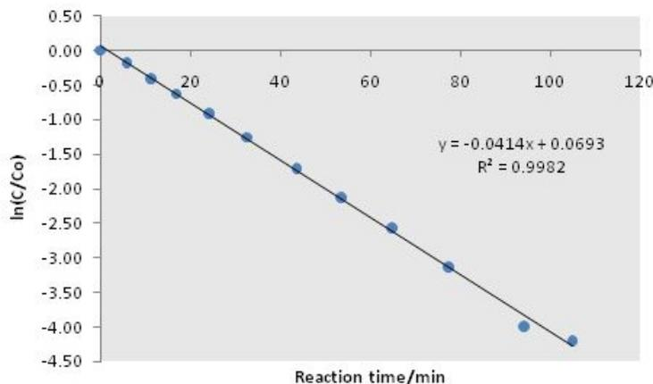
**Figure 4.12:** A plot of  $\ln(C_{\text{TCE}}/C_0)$  versus time.
