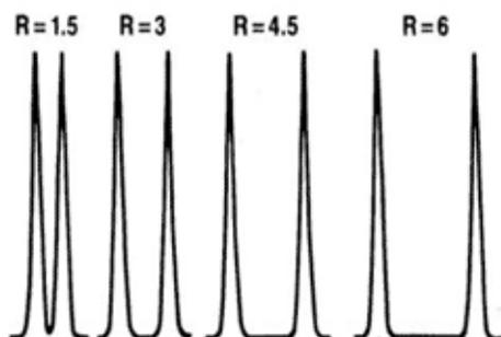
**Figure 4.5:** Different separation resolutions. Adapted from <http://www.gchelp.tk>
