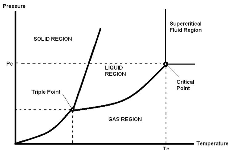
Figure 4.21: Schematic representation of an idealized phase diagram.
