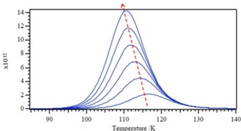
**Figure 4.18:** A simulated second-order TPD experiment: A second-order reaction between adsorbates and surface. Values of  $T_m$  decrease as the initial coverage  $\theta$  increases from  $1.0 \times 10^{13}$  to  $6.0 \times 10^{13} \text{ cm}^{-2}$ ;  $E_a = 30 \text{ KJ/mol}$ ;  $\beta = 1.5 \text{ }^\circ\text{C/s}$ ;  $A = 1 \times 10^{-1}$ .
