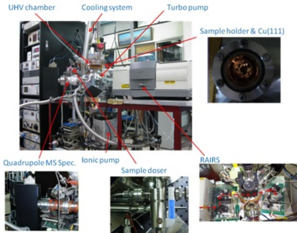
**Figure 4.14:** A typical TPD apparatus composed of a UHV chamber equipped with a series of pumping systems, cooling system, sample dosing system as well as surface detection instruments including a quadrupole MS Spectrometer and a reflection absorption infra red spectrometer (RAIRS).
