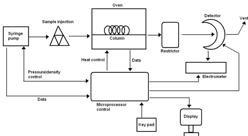
**Figure 4.22:** Scheme of a supercritical fluid chromatography instrument. Adapted from D. A. Skoog and J. J. Leary, *Principles of Instrumental Analysis*, Saunders College Publishing, Philadelphia (1992).
