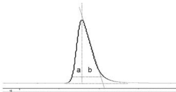
**Figure 4.8:** Scheme for the symmetry of a peak. Adapted from <http://www.gchelp.tk>
