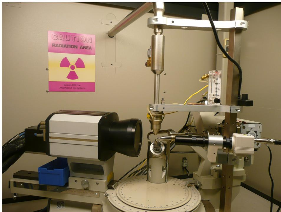
**Figure 6.34:** Single crystal X-ray diffractometer with a CCD detector. The incident beam is generated and delivered through the silver apparatus on the right side of the sample, and the detector is the large black camera to the left of the sample.
