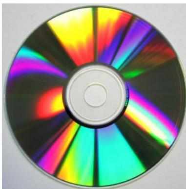
**Figure 6.30:** The rainbow effects caused by visible light striking the grooves of a compact disc (CD).
