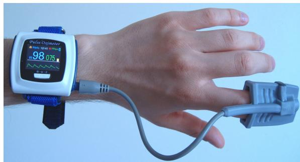
**Figure 7.27** A pulse oximeter is an apparatus that measures the amount of oxygen in blood. Oximeters can be used to determine a person's metabolic rate, which is the rate at which food energy is converted to another form. Such measurements can indicate the level of athletic conditioning as well as certain medical problems. (credit: UusiAjaja, Wikimedia Commons)
