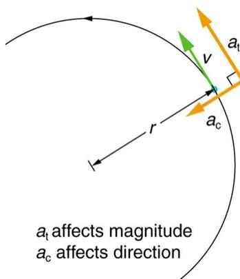
**Figure 10.5** Centripetal acceleration  $a_c$  occurs as the direction of velocity changes; it is perpendicular to the circular motion. Centripetal and tangential acceleration are thus perpendicular to each other.
