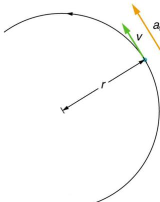
**Figure 10.4** In circular motion, linear acceleration  $a$ , occurs as the magnitude of the velocity changes:  $a$  is tangent to the motion. In the context of circular motion, linear acceleration is also called tangential acceleration  $a_t$ .
