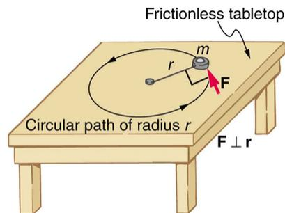
**Figure 10.11** An object is supported by a horizontal frictionless table and is attached to a pivot point by a cord that supplies centripetal force. A force  $F$  is applied to the object perpendicular to the radius  $r$ , causing it to accelerate about the pivot point. The force is kept perpendicular to  $r$ .
