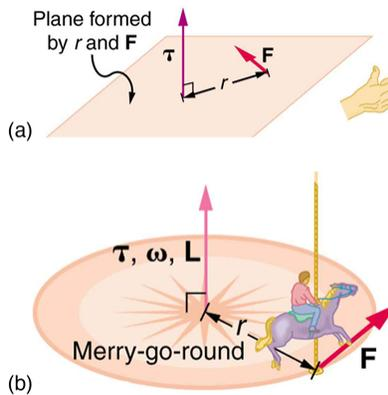
**Figure 10.29** In figure (a), the torque is perpendicular to the plane formed by  $r$  and  $\mathbf{F}$  and is the direction your right thumb would point to if you curled your fingers in the direction of  $\mathbf{F}$ . Figure (b) shows that the direction of the torque is the same as that of the angular momentum it produces.
