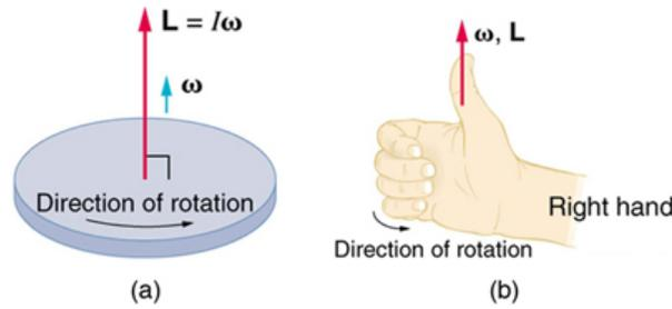
**Figure 10.28** Figure (a) shows a disk is rotating counterclockwise when viewed from above. Figure (b) shows the right-hand rule. The direction of angular velocity  $\boldsymbol{\omega}$  size and angular momentum  $\mathbf{L}$  are defined to be the direction in which the thumb of your right hand points when you curl your fingers in the direction of the disk's rotation as shown.
