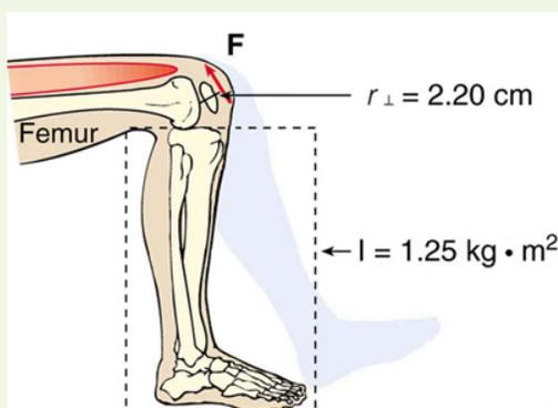
**Figure 10.22** The muscle in the upper leg gives the lower leg an angular acceleration and imparts rotational kinetic energy to it by exerting a torque about the knee.  $\mathbf{F}$  is a vector that is perpendicular to  $r$ . This example examines the situation.
