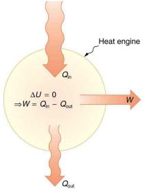
Figure 15.7 Schematic representation of a heat engine, governed, of course, by the first law of thermodynamics. It is impossible to devise a system where  $Q_{out} = 0$ , that is, in which no heat transfer occurs to the environment.
