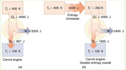
Figure 15.35 (a) A Carnot engine working at between 600 K and 100 K has 4000 J of heat transfer and performs 3333 J of work. (b) The 4000 J of heat transfer occurs first irreversibly to a 250 K reservoir and then goes into a Carnot engine. The increase in entropy caused by the heat transfer to a colder reservoir results in a smaller work output of 2400 J. There is a permanent loss of 933 J of energy for the purpose of doing work.
