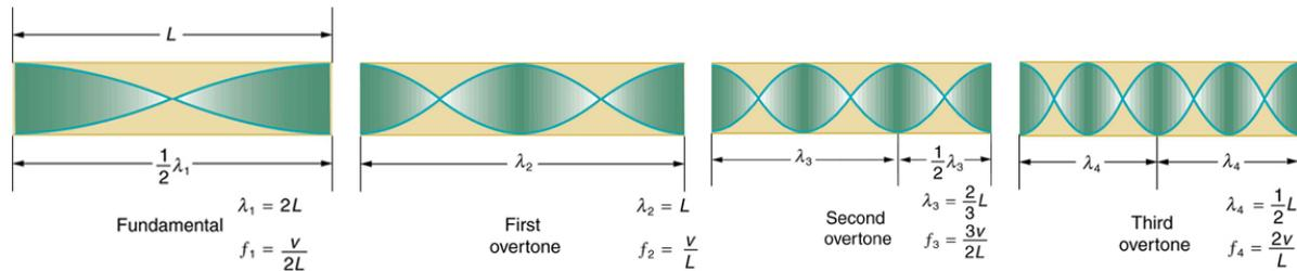
**Figure 17.31** The resonant frequencies of a tube open at both ends are shown, including the fundamental and the first three overtones. In all cases the maximum air displacements occur at both ends of the tube, giving it different natural frequencies than a tube closed at one end.
