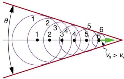
**Figure 17.17** Sound waves from a source that moves faster than the speed of sound spread spherically from the point where they are emitted, but the source moves ahead of each. Constructive interference along the lines shown (actually a cone in three dimensions) creates a shock wave called a sonic boom. The faster the speed of the source, the smaller the angle  $\theta$ .
