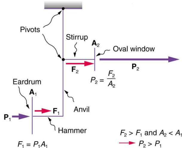
**Figure 17.40** This schematic shows the middle ear's system for converting sound pressure into force, increasing that force through a lever system, and applying the increased force to a small area of the cochlea, thereby creating a pressure about 40 times that in the original sound wave. A protective muscle reaction to intense sounds greatly reduces the mechanical advantage of the lever system.
