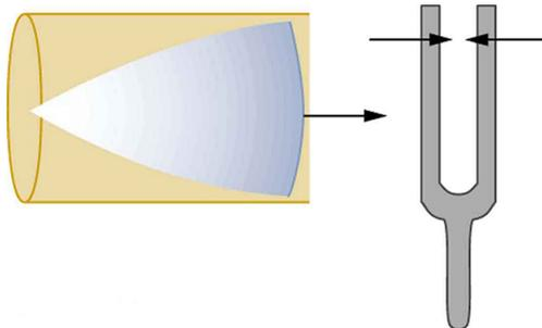
**Figure 17.26** Resonance of air in a tube closed at one end, caused by a tuning fork. A graph of air displacement along the length of the tube shows none at the closed end, where the motion is constrained, and a maximum at the open end. This standing wave has one-fourth of its wavelength in the tube, so that  $\lambda = 4L$ .
