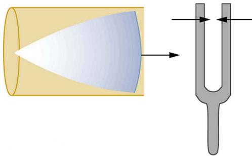
**Figure 17.25** Resonance of air in a tube closed at one end, caused by a tuning fork. If the length of the tube  $L$  is just right, the disturbance gets back to the tuning fork half a cycle later and interferes constructively with the continuing sound from the tuning fork. This interference forms a standing wave, and the air column resonates.
