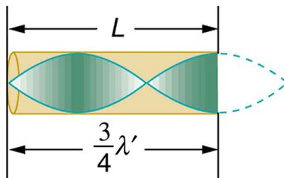
**Figure 17.28** Another resonance for a tube closed at one end. This has maximum air displacements at the open end, and none at the closed end. The wavelength is shorter, with three-fourths  $\lambda'$  equaling the length of the tube, so that  $\lambda' = 4L/3$ . This higher-frequency vibration is the first overtone.
