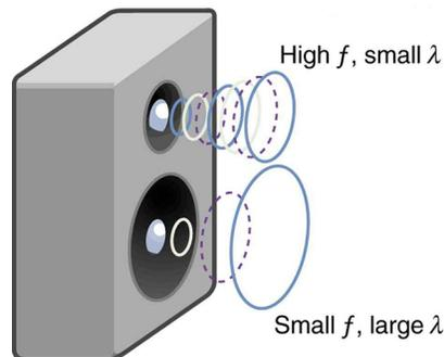
**Figure 17.11** Because they travel at the same speed in a given medium, low-frequency sounds must have a greater wavelength than high-frequency sounds. Here, the lower-frequency sounds are emitted by the large speaker, called a woofer, while the higher-frequency sounds are emitted by the small speaker, called a tweeter.
