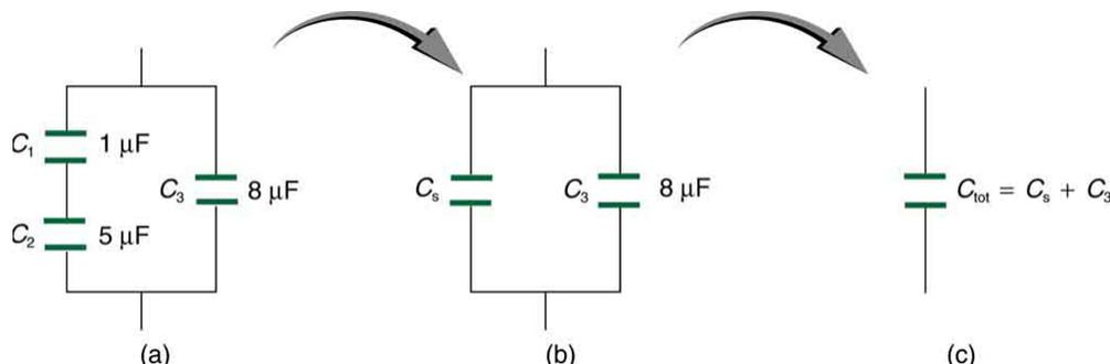
**Figure 19.23** (a) This circuit contains both series and parallel connections of capacitors. See **Example 19.10** for the calculation of the overall capacitance of the circuit. (b)  $C_1$  and  $C_2$  are in series; their equivalent capacitance  $C_s$  is less than either of them. (c) Note that  $C_s$  is in parallel with  $C_3$ . The total capacitance is, thus, the sum of  $C_s$  and  $C_3$ .
