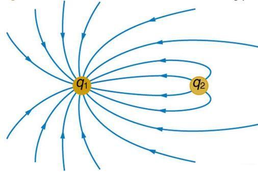
**Figure 19.28** The electric field near two charges.
