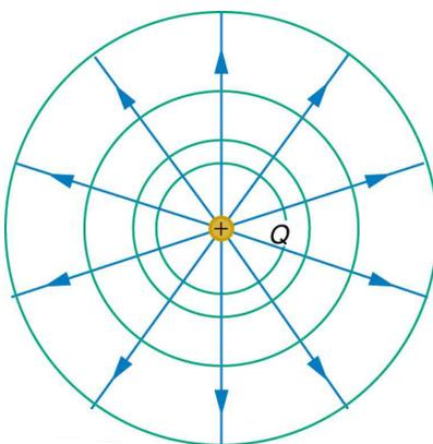
**Figure 19.8** An isolated point charge  $Q$  with its electric field lines in blue and equipotential lines in green. The potential is the same along each equipotential line, meaning that no work is required to move a charge anywhere along one of those lines. Work is needed to move a charge from one equipotential line to another. Equipotential lines are perpendicular to electric field lines in every case.
