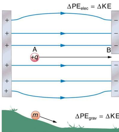
**Figure 19.2** A charge accelerated by an electric field is analogous to a mass going down a hill. In both cases potential energy is converted to another form. Work is done by a force, but since this force is conservative, we can write  $W = -\Delta PE$ .
