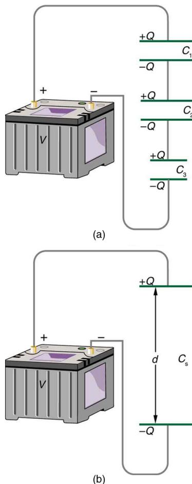
**Figure 19.21** (a) Capacitors connected in series. The magnitude of the charge on each plate is  $Q$ . (b) An equivalent capacitor has a larger plate separation  $d$ . Series connections produce a total capacitance that is less than that of any of the individual capacitors.
