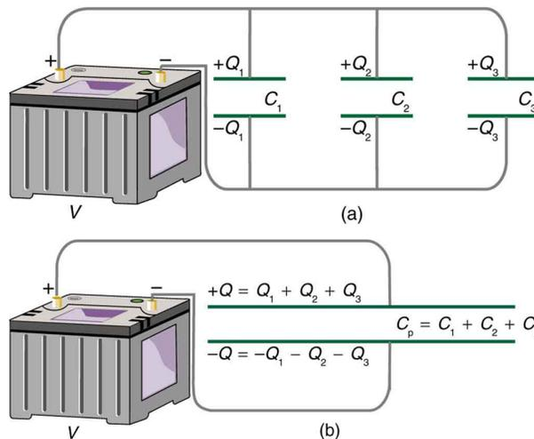
**Figure 19.22** (a) Capacitors in parallel. Each is connected directly to the voltage source just as if it were all alone, and so the total capacitance in parallel is just the sum of the individual capacitances. (b) The equivalent capacitor has a larger plate area and can therefore hold more charge than the individual capacitors.
