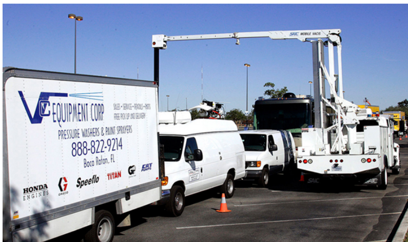
Figure 32.2 Customs officers inspect vehicles using neutron irradiation. Cars and trucks pass through portable x-ray machines that reveal their contents. (credit: Gerald L. Nino, CBP, U.S. Dept. of Homeland Security)
