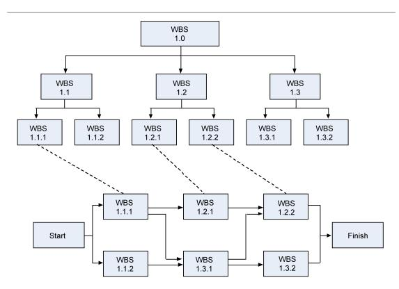
Figure 12: The relationship between the work breakdown structure (WBS) and the network diagram.
