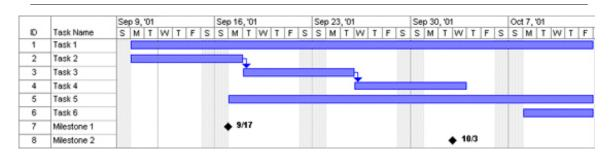
Figure 5: An example of a Gantt chart showing the relationship between a series of tasks.
