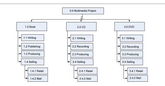
Figure 5: An example of a work breakdown structure (WBS) based on project deliverable.
