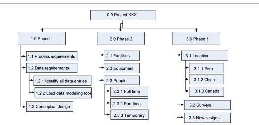
Figure 6: An example of a work breakdown structure (WBS) based on project phase.
