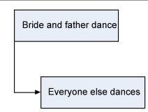
Figure 10: A lag means making sure that one task waits a while before it gets started.
